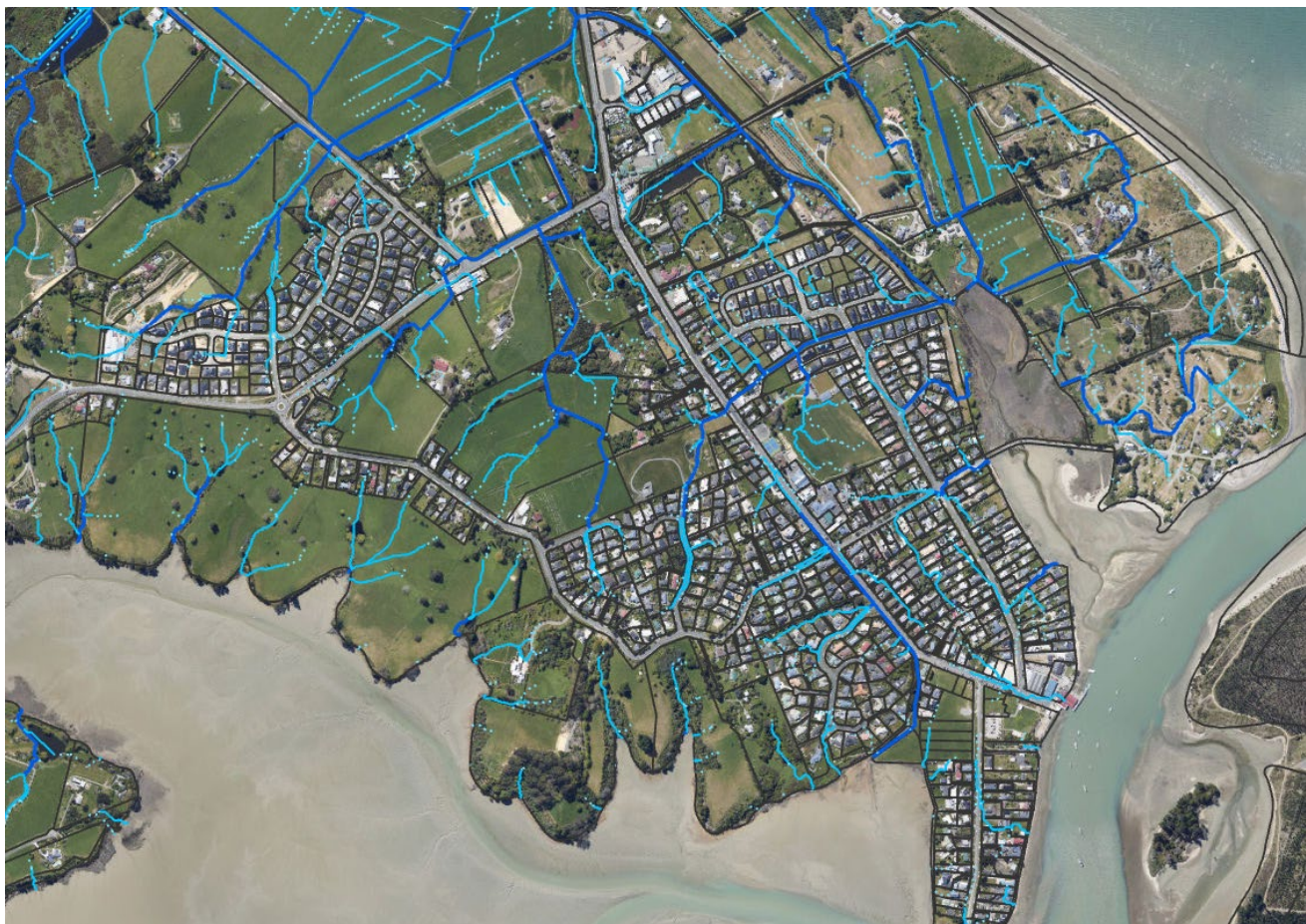
Figure 10: Māpua modelled overland flows (from LiDAR)
