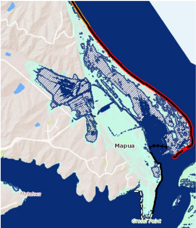
Figure 11: Māpua coastal inundation bathtub model
