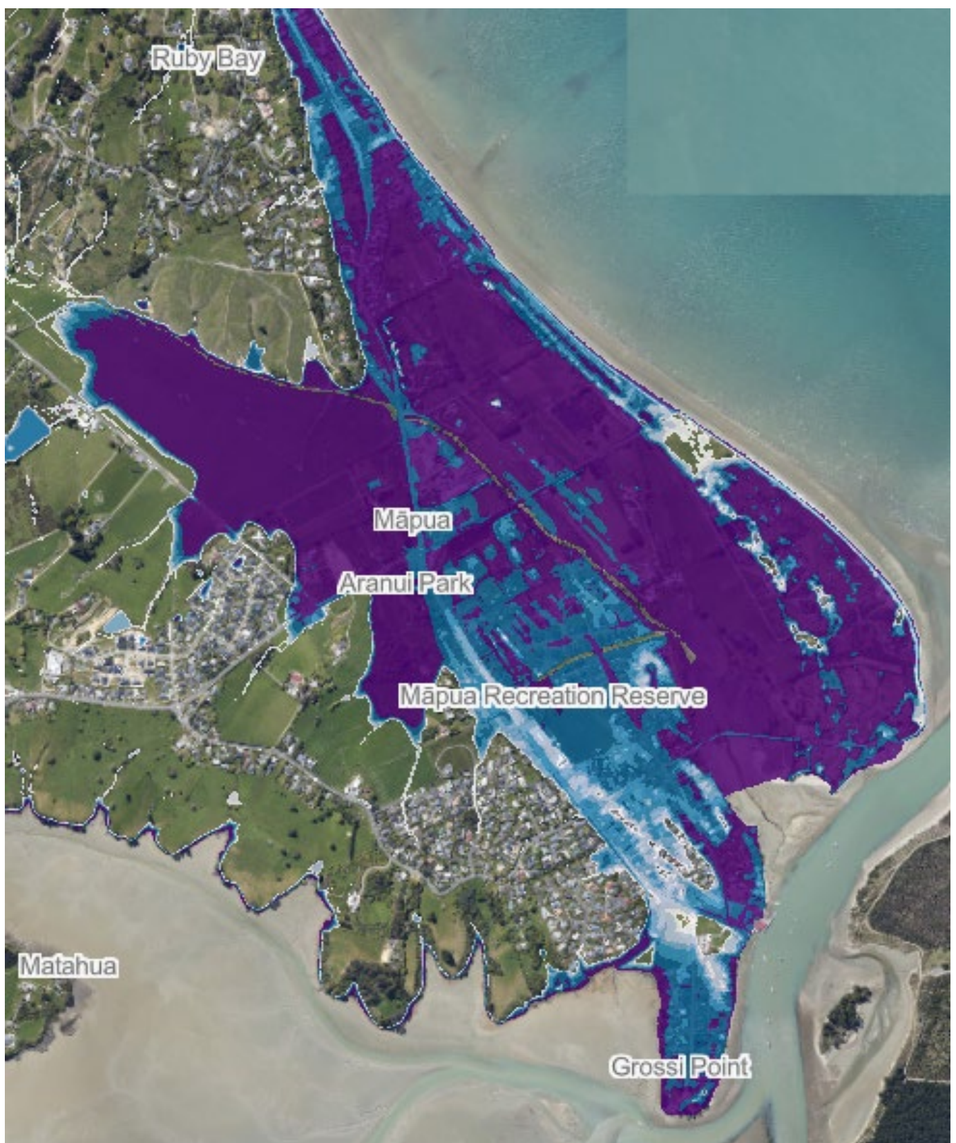
Figure 13: Māpua flooding from 1% AEP future rainfall with sea level rise and coastal overtopping
