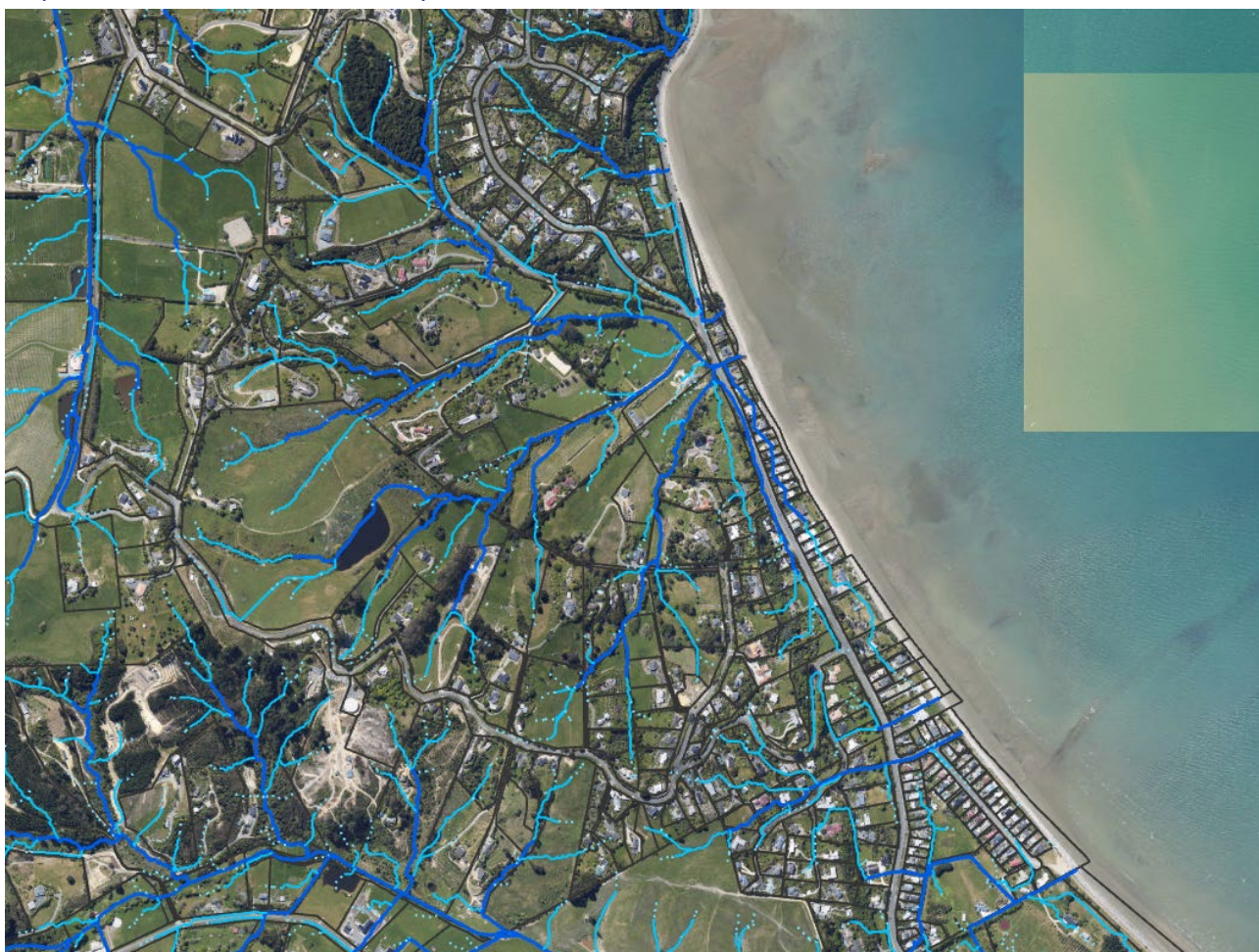
Figure 9: Ruby Bay modelled overland flows (from LiDAR)
