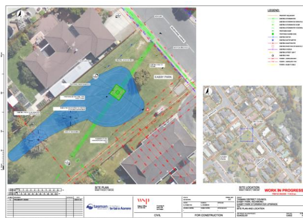
Proposed location of shallow stormwater detention feature at Easby Park
