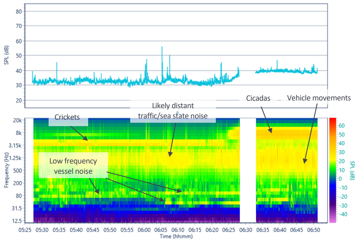
Figure 13: 84 Selwyn Street (16 Feb): time trace and spectrogram in A-weighted levels
